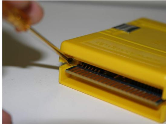
With the opening in the Chameleon case for the mini-DIN connector, the left half of the case top is fairly weak. It is unlikely to break if you do not use extreme force (polycarbonate is very flexible), but it's still a good idea to be as gentle as possible. We therefore recommend to open the right side of the case first:
